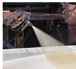
With 3M™ Scotch-Weld™ Cylinder Spray Adhesive Foam Fast 74NF, a fast light coat bonds quilted fabric to solid core mattress. High coverage reduces application cost. Foam-tearing strength prevents cover spin.
