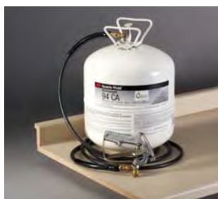
For HPL countertop assembly, 3M™ Scotch-Weld™ Cylinder Spray Adhesive 94CA dries quickly to reach postformable strength in 1-5 minutes. 1-15 minute open time provides flexibility in assembly speed. Formulated specifically with low telegraphing for thin veneers and glossy laminates.
